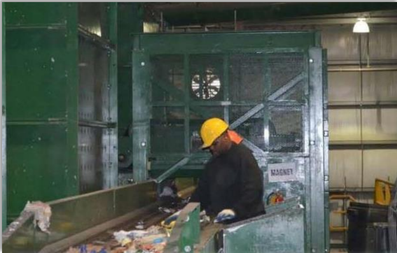
Conveyor leading up to the magnet (inside the green cage behind the worker).
