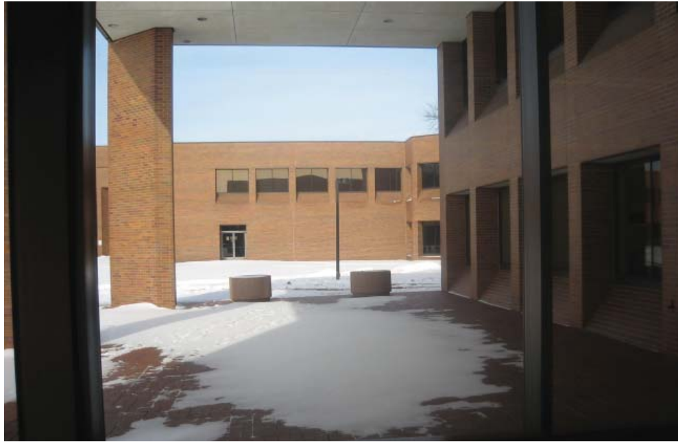
Unused Outdoor Patios. Patios are inhospitable. Tall canopies create windy conditions resulting in under used outdoor spaces.
