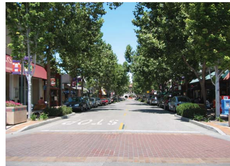
Streets lined with trees create a perceived narrowing of the roadway therefore slowing traffic.
